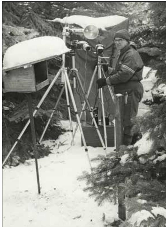
Isidor Jeklin’s setup for winter photography consisted of two cameras of different focal lengths that were both connected to a high-speed strobe, winter 1983.
