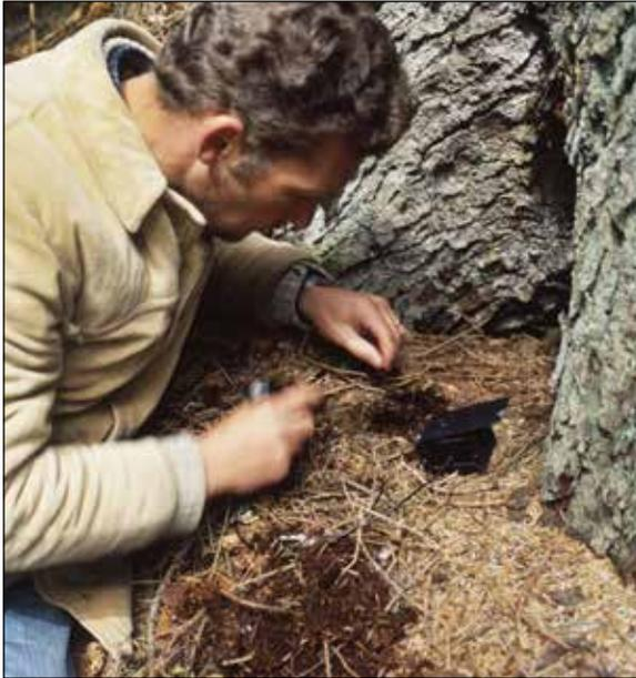
Me installing a photo-electric triggering device at the burrow of an Ancient Murrelet on Reef Island, Haida Gwaii, 1985.
